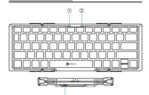
① Power/Charging/Low Battery/ Bluetooth Pairing Indicator Power indicator: when unfold the keyboard, the indicator will turn green for 3 seconds then to be off
