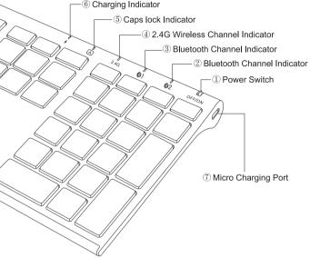
① Power Switch: slide right to turn on and left to turn off.
